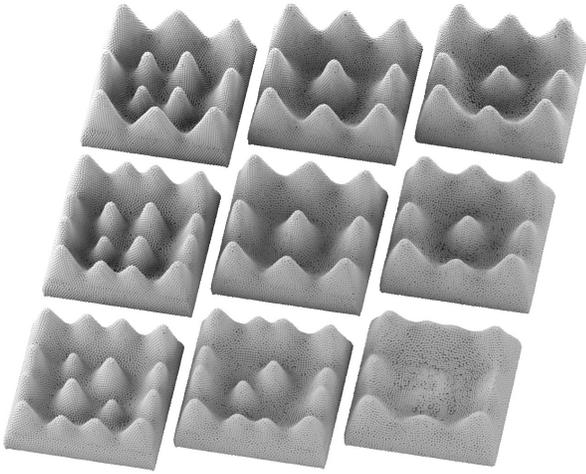
Fig. 4: Illustration of varying surface tension along the horizontal axis (0.25, 0.5, 1.0) and varying magnetic field strength ( $1.2 \cdot 10^5$  A/m,  $1.3 \cdot 10^5$  A/m,  $1.4 \cdot 10^5$  A/m) along the vertical axis. The box size is  $0.05 \text{ m} \times 0.05 \text{ m} \times 0.015 \text{ m}$ .
