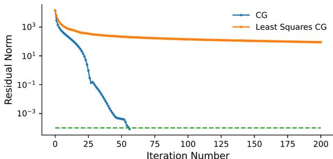
Fig. 9: The residual norm between our newly implemented solver compared to the previous one of Huang et al. [21]. The blue curve corresponds to the new conjugate gradient solver while the orange curve corresponds to the least squares conjugate gradient solver [21]. Here, we are solving for the magnetic field of a sphere with radius of 2 cm. The susceptibility is set to be 500.
