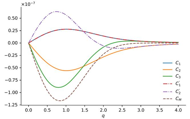
Fig. 1: Illustration of the new curves  $C_1, C_2, C_3$  in our current loop model, and the old curves  $C'_1, C'_2$  from Huang et al. [21].  $C_M$  corresponds to the extra term induced by the second integration of Eq. (29).
