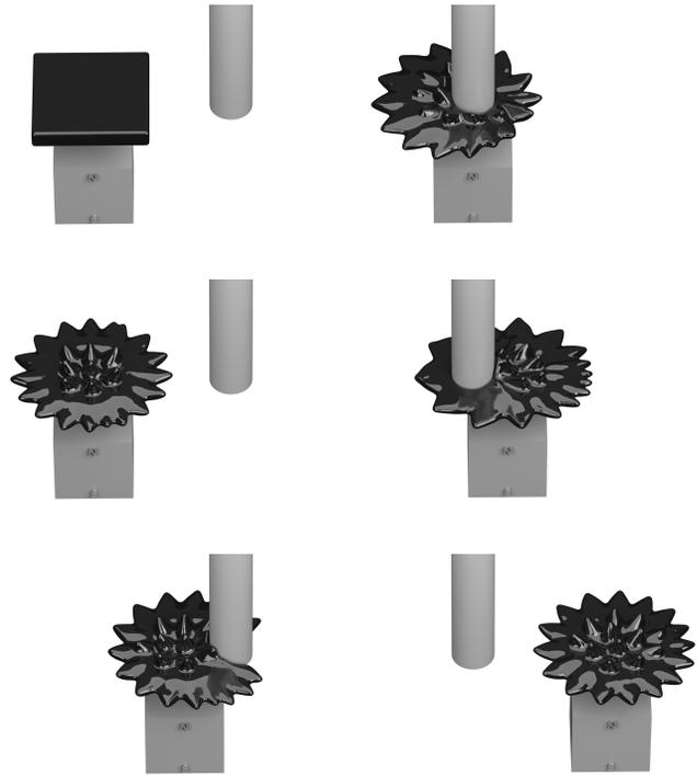
Fig. 6: The time sequence of this experiment is shown in an N-shape direction. The cube magnet leads to a magnetic field direction along the vertical axis. The edge length of the cube is 4 cm.
