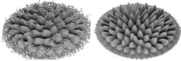
(a) When employing a dipole field, the importance of our fitted force model is even more evident compared to the case of the constant magnetic field shown before in Figure 10b: the center force model (left) leads to unstable results compared to the fitted force model (right).
