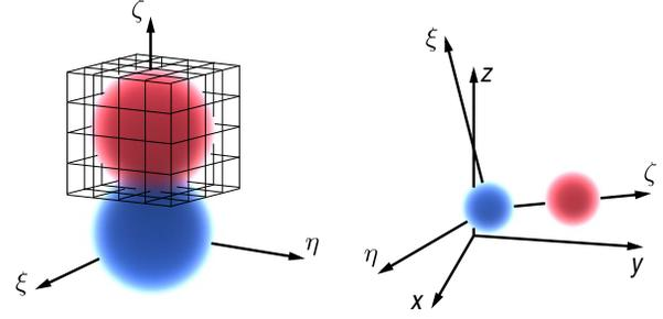
Fig. 5. Illustration of measuring the force from the source kernel (blue) to the target kernel (red) in the rotated coordinates  $(\xi, \eta, \zeta)$  (left) and rotated coordinates  $(\xi, \eta, \zeta)$  embedded in world coordinates  $(x, y, z)$  (right).
