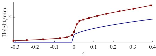
Fig. 9. Illustration of the dependence of the average height of the formed spikes on the bifurcation parameter  $\epsilon$ . Our simulation (red squares) successfully reproduces the qualitative trend shown in real data (blue curve; [Gollwitzer et al. 2007], Figure 12) while the height of the spikes differs due to different surface tension strengths. The formation of the spikes can precisely be observed around  $\epsilon = 0$  in the simulation and in reality.
