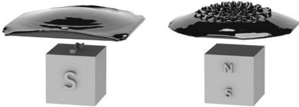
Fig. 13. If the magnetic field lines are oriented almost in parallel to the ferrofluid’s surface, no spikes can be observed (left). An appropriate rotation of the magnet causing a proper reorientation of the field lines leads to the presence of spikes (right).
