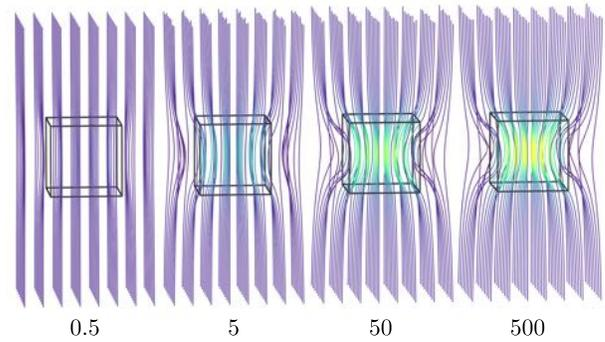
Fig. 3. Illustration of the field lines of a constant vertical magnetic field under the influence of cubes with different susceptibility  $\chi$ . The susceptibility set to  $\chi = 0.5, 5, 50, 500$  (from left to right). Typical ferrofluids have a susceptibility between 1 and 5 [Rosenweig 1987]. The field lines are generated by advancing tracing particles along the magnetic flux density direction  $\mathbf{B}$ . Please note that four independent fields are plotted.
